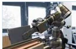
The key element of the mobile robot is a lightweight arm from SCHUNK. For being able to grip books, a mechatronic parallel gripper from SCHUNK is used.
